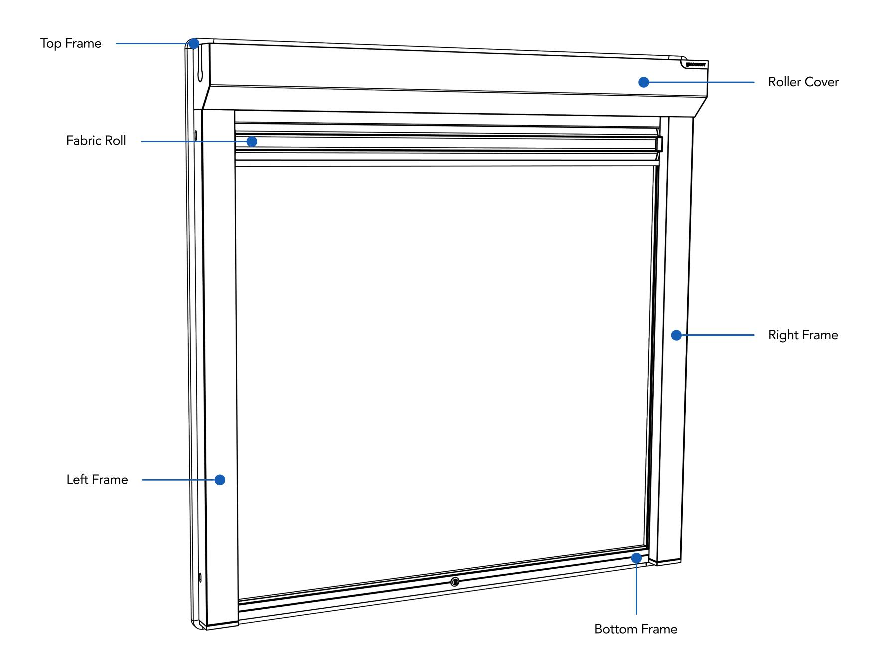
**Assembled Frame** Isometric View
